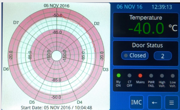
LCD Screen Display for Plasma Storage Cabinet (-40°C)s
